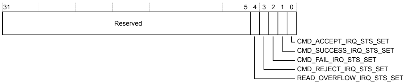
Figure 3-8 IRQ_STATUS_SET register bit assignments
