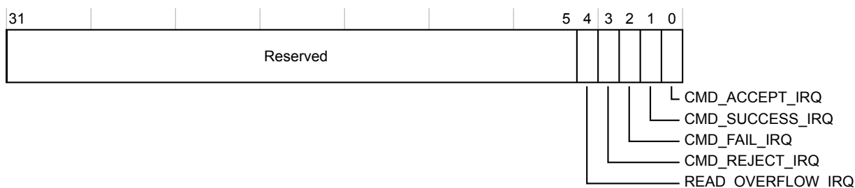
Figure 3-10 IRQ_MASKED_STATUS register bit assignments
